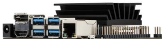
Side view of the Jetson Nano Developer Kit showing most of the available ports. ( : NVIDIA)
